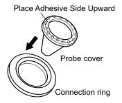
3. Insert the probe into the probe cover on the connection ring until it clicks.
